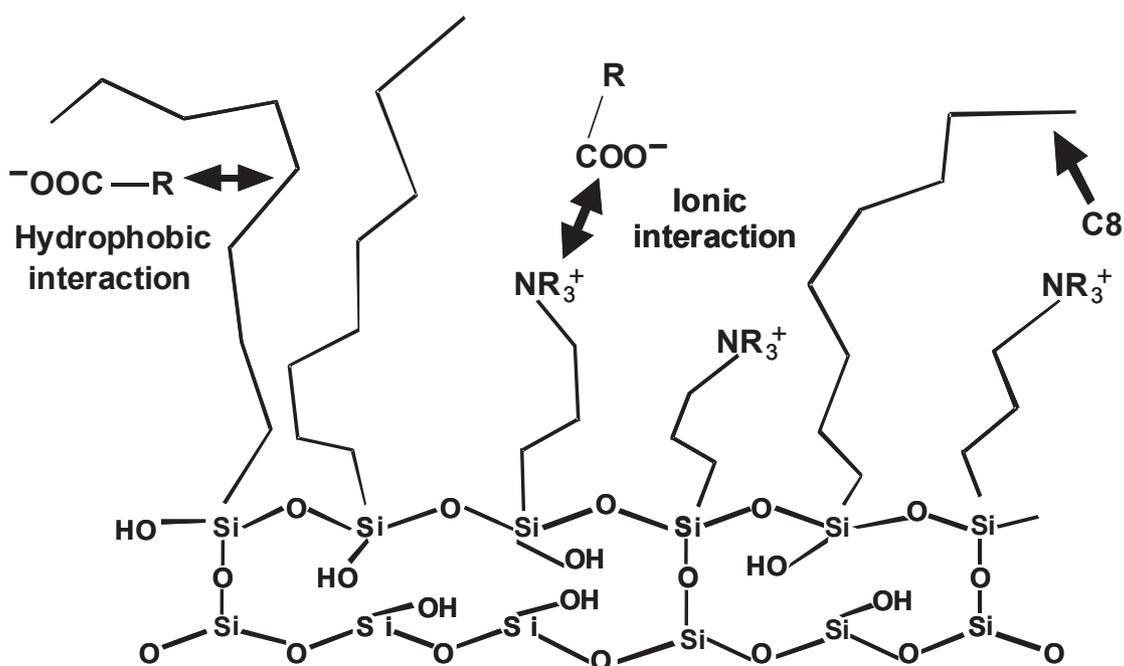
**Figure 1.** Multiple interactions on ISOLUTE HAX mixed-mode columns
