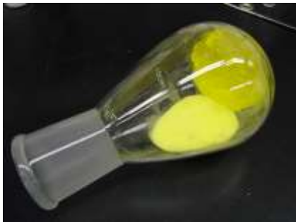
Preadsorption on silica gel (3 g)
