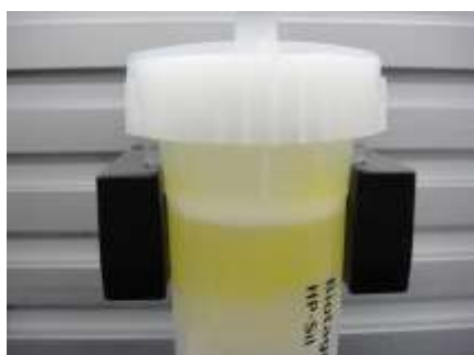
Band formed when chromatography was run immediately after pretreatment.
