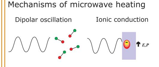
The phase difference between the field and dipole polarizations causes energy to be lost from the dipole. The energy is converted to heat by random collisions. The electric field component of the wave forces the charged particles in the material to move back and forth. The energy is again converted to heat by random collisions.
