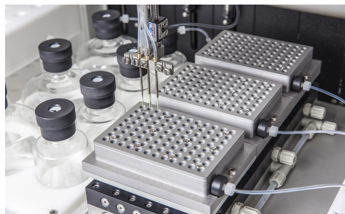
Syro II parallel peptide synthesizer. Configured with optional Tip Synthesis reactor blocks and inert gas.
