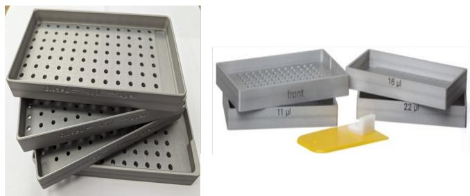
Figure 2. Resin loading tools for 96 x 2 mL heating blocks (left) and 0.4 mL Tip reactor vials (right).
